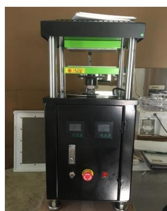
A rosin press consists of two heated plates which are pressed together at high pressure (typically between 300 to 600 psi) to convert hashish into rosin. This process is typically considered non-volatile manufacturing.
