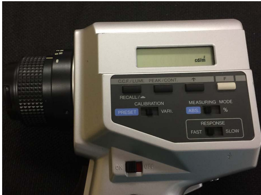
Figure 18: Minolta LS-100 meter
