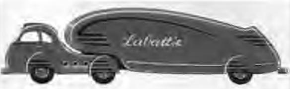
both front and rear, rather than being rounded to a flat bottom surface. This makes the front and rear more similar, the front less snubbed and the rear less sloped. The trailer features a stainless steel 'dorsal fin', principally for ornamentation.
