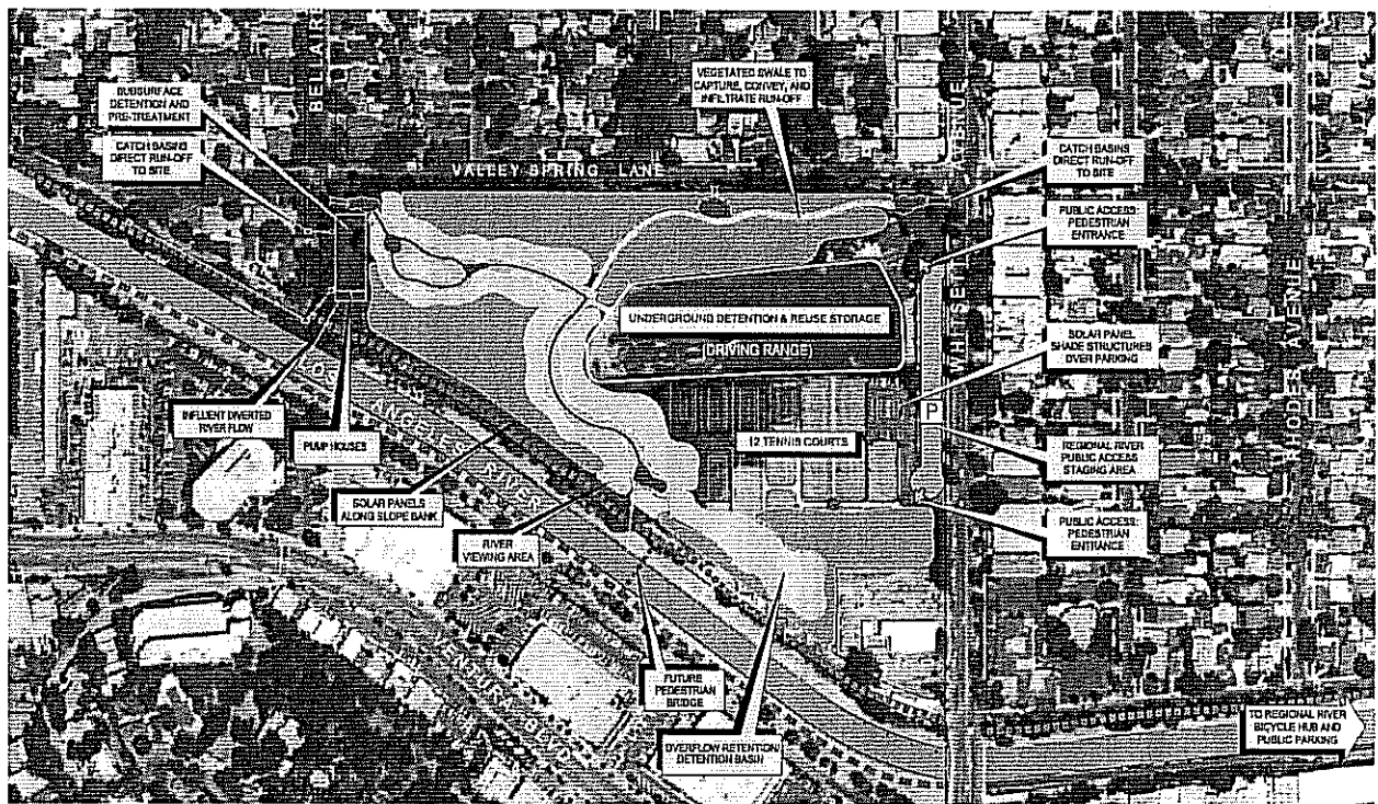
L.A. River Natural Park: Water Quality Improvement Components Concept Plan. Developed by P50MA5
