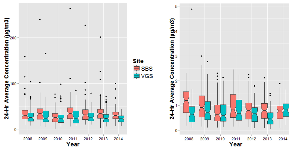
Figure 1. Notched box-whisker plot of daily 24-hr average concentrations of PM 10 (left) and BC (right) at Sunshine Canyon Landfill (SBS) and Van Gogh (VGS) during fall quarters in 2008 to 2014.
