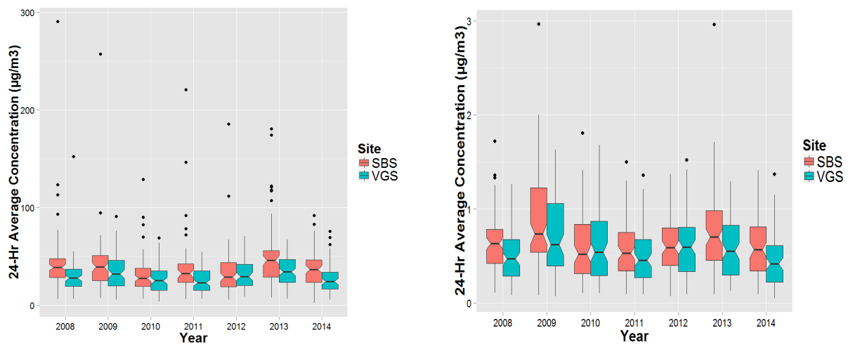
Figure 4-1. Notched box-whisker plot of daily 24-hr average concentrations during spring season at Sunshine Canyon Landfill (SBS) and Van Gogh (VGS) in years 2008 to 2014 for PM 10 (left) and BC (right).
