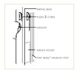
**Step 6:** Tie the end of the twine to the new sash cord and then pull the fishing weight until you can see the sash cord in the pocket.
