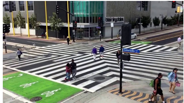
A pedestrian “scramble” crosswalk with bicycle and pedestrian safety features, Santa Monica
