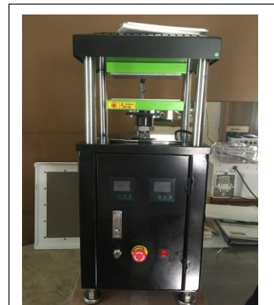
A rosin press consists of two heated plates which are pressed together at high pressure (typically between 300 to 600 psi) to convert hashish into rosin. This process is typically considered non-volatile manufacturing.
