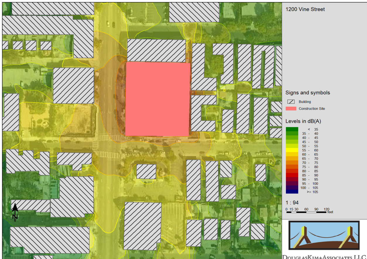
Figure 6-2 Construction Noise Sound Contours
