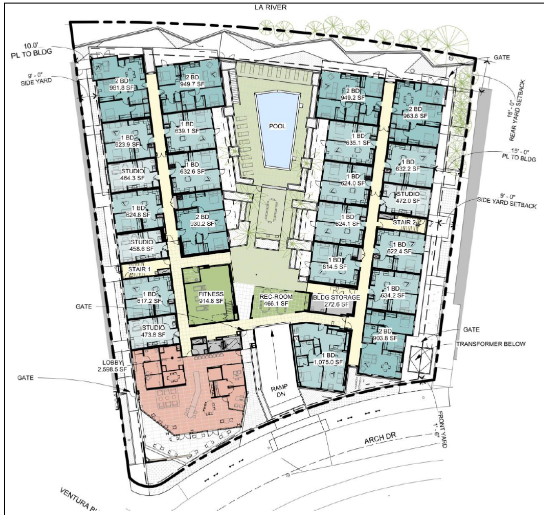
Figure 4: Ground Floor with lobby, front deck, pool deck, amenity rooms, and dwelling units.
