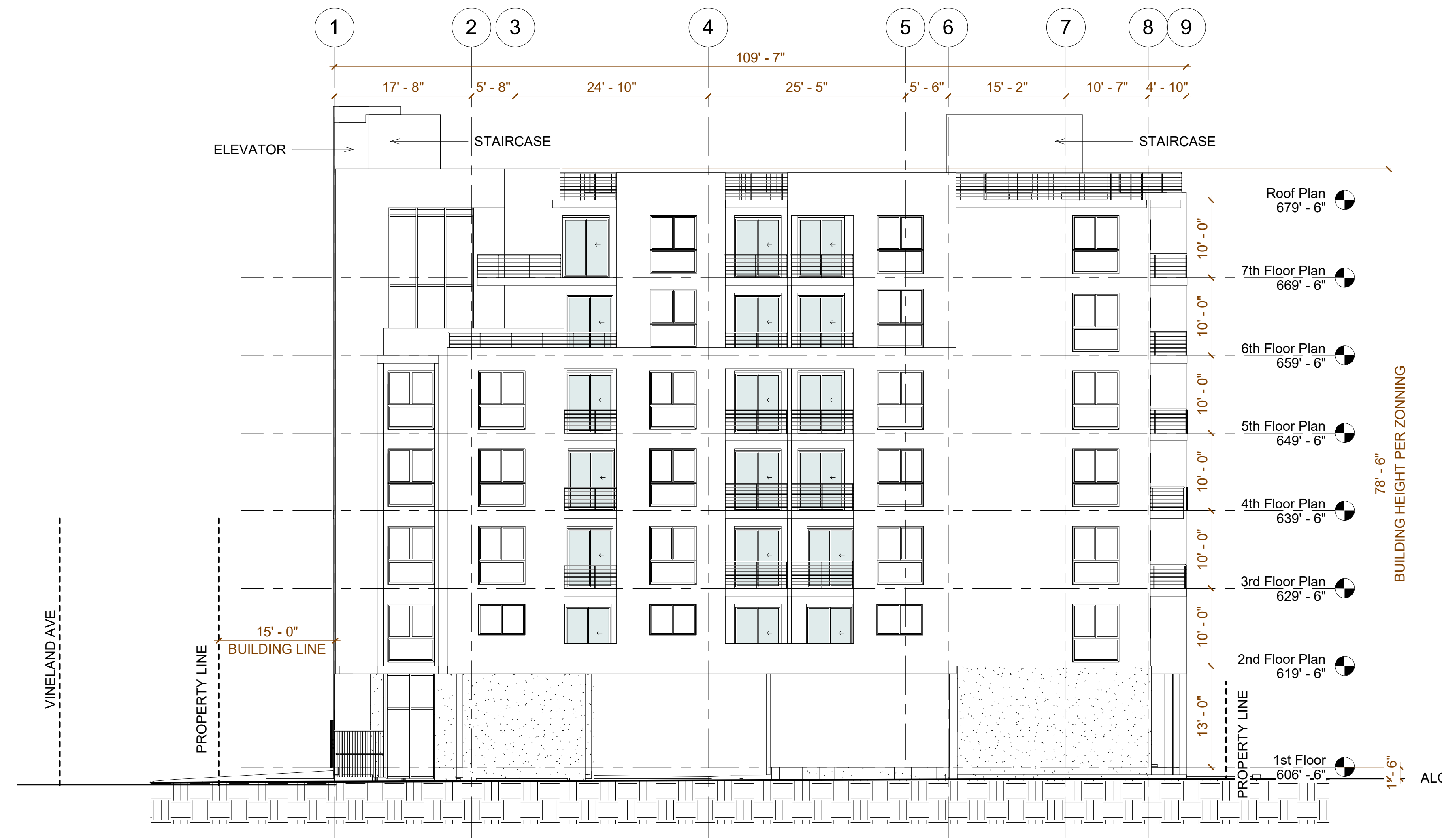
① SOUTH ELEVATION 1" = 10'-0"
