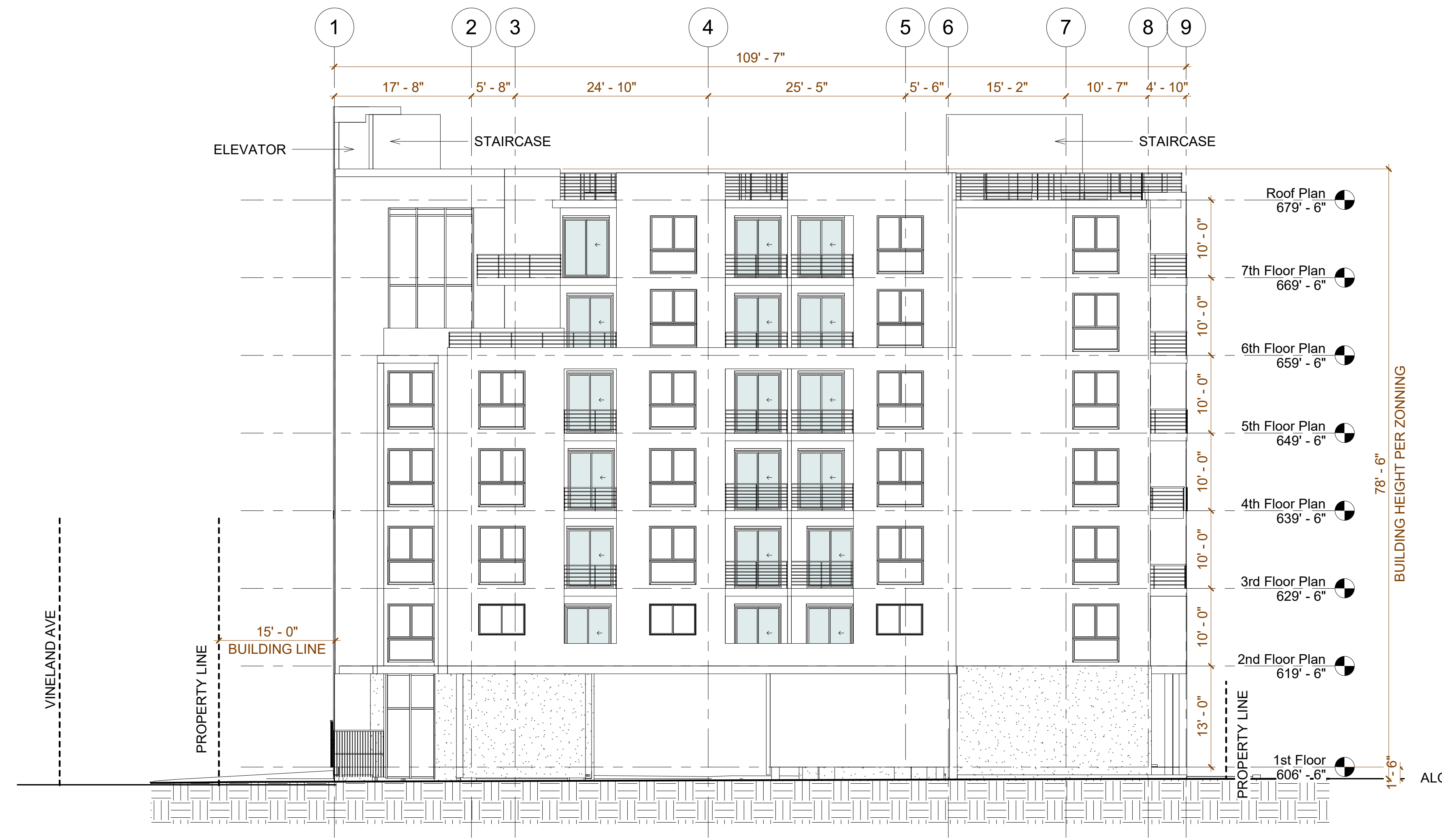
① SOUTH ELEVATION 1" = 10'-0"
